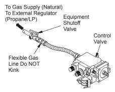
Figure 32 - Connecting Flexible Gas Line to Control Valve
